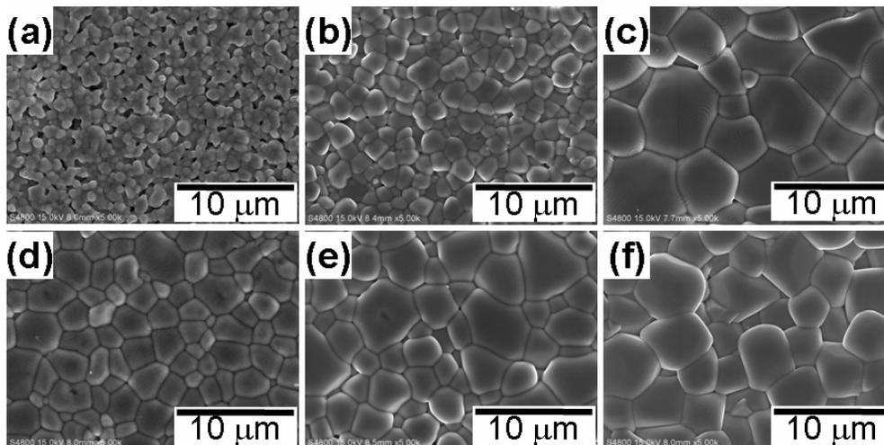
**Fig. 3.** SEM micrographs of thermally etched surfaces of the pure PMNZT ceramics sintered at (a) 950, (b) 1050, (c) 1200°C, and samples with the addition of 0.1 wt% CuO sintered at (d) 950, (e) 1050, (f) 1200°C for 4 h in air.
