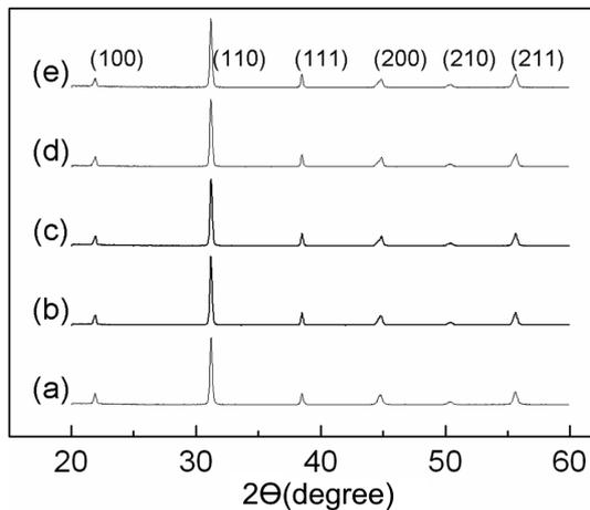
**Fig. 1.** X-ray diffraction patterns of the PMNZT ceramics with (a) 0, (b) 0.05 (c) 0.1 (d) 0.2 (e) 0.3 wt% of CuO additions sintered at 1050°C.
