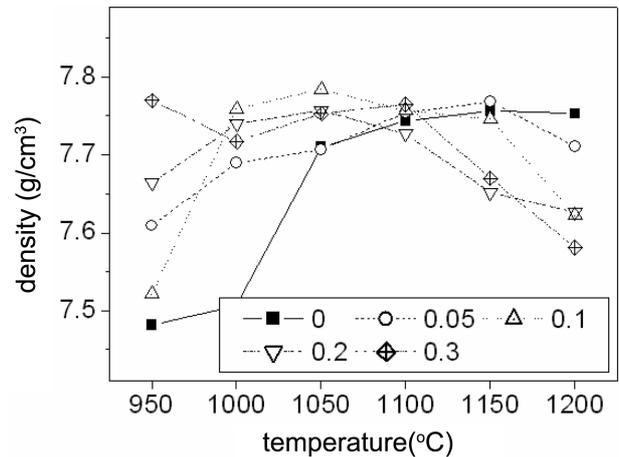
**Fig. 2.** Densities as a function of sintering temperature for PMNZT ceramics with various CuO additions.
