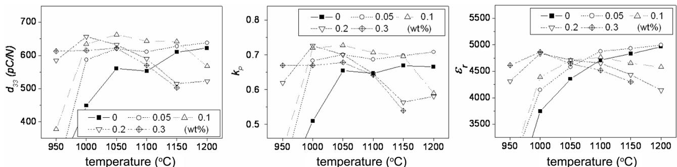
**Fig. 4.** Piezoelectric coefficients ( $d_{33}$ ), planar mode electromechanical coupling coefficients ( $k_p$ ), and dielectric constants ( $\epsilon_r$ ) of pure and CuO added PMNZT ceramics sintered for 4 h in air at various temperatures.
