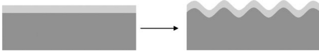
Fig. 1. Schematic drawing for the buckling of a thin film on a compliant substrate. [30]
