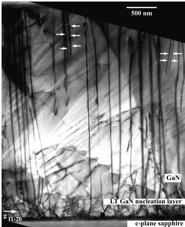
Fig. 17. Weak beam cross-sectional image of a fully grown GaN epitaxial layer obtained using the (11\bar{2}0) reflection.
